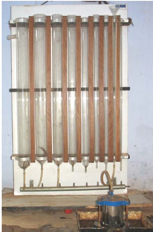
Plate 3.6 Falling head permeability test
