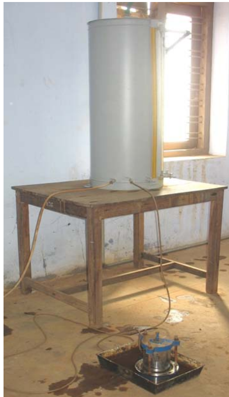
Plate 3.5 Constant head permeability test
