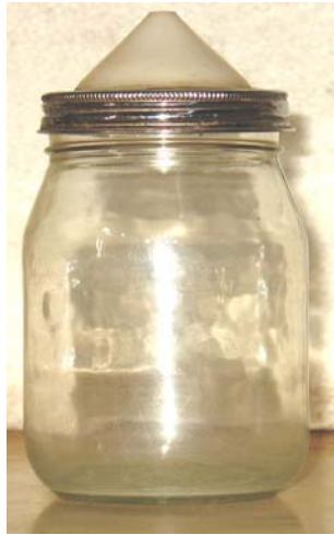
Plate 3.4 Pycnometer for specific gravity determination
