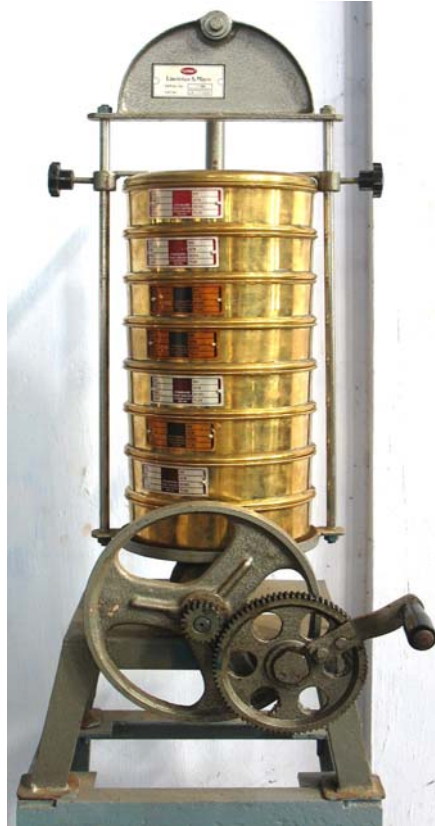
Plate 3.2 Sieve analysis setup
