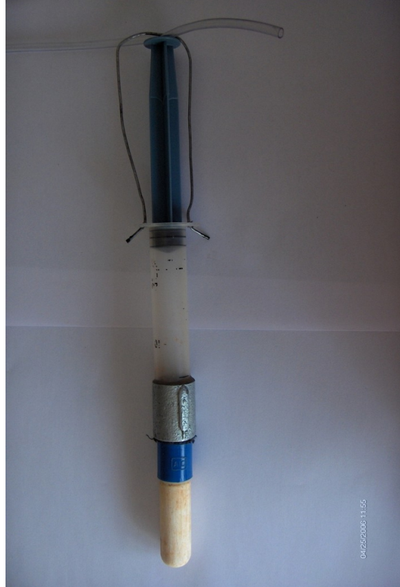
Plate 1. Arrangement of tension-emitter with a single porous cup and piston
