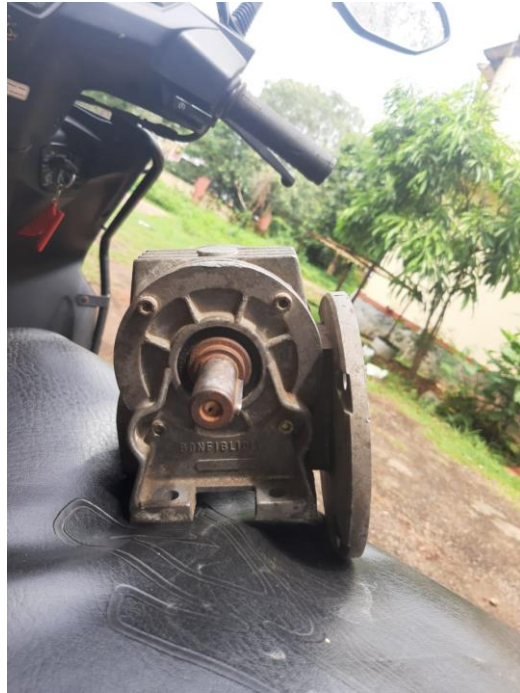
Plate 3.4 Reduction gear box (output shaft)
