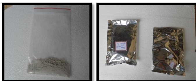
Plate 4.3 Packaged pseudostem juice powder samples in LDPE pouches and aluminium foil pouches
