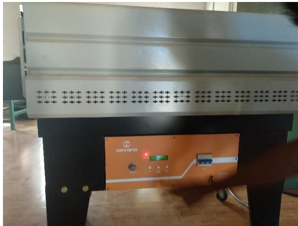
Plate 3.5 Shrink wrap packaging machine
