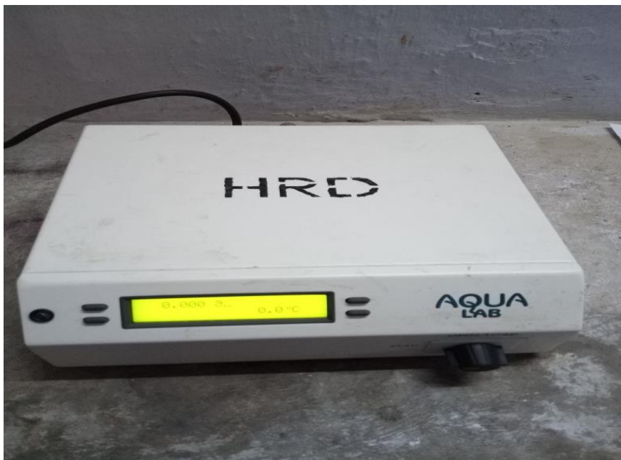
Plate 3.2 Aqualab Water Activity Meter
