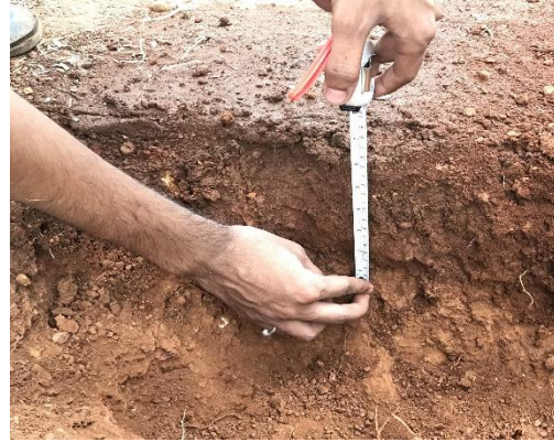
Plate 3.17 Wetted Depth of Bulb
