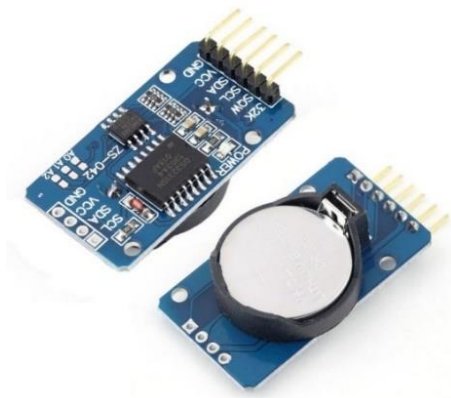
Plate 3.11 Real Time Clock
