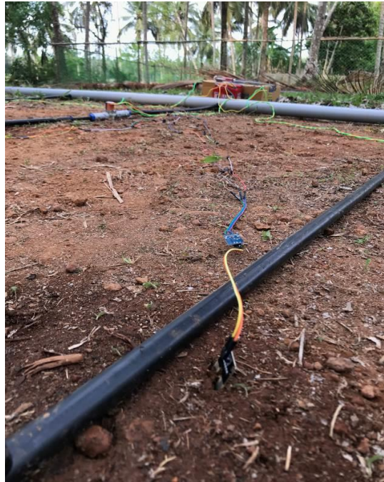
Plate 3.22 Position of soil moisture sensor
