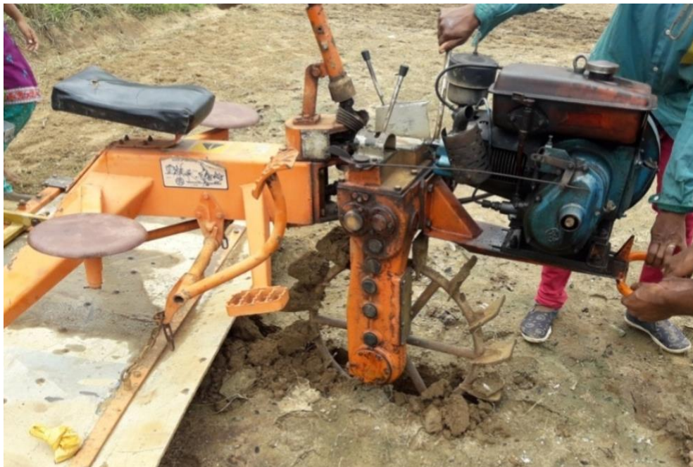
Fig. 4.11 Drive wheel stuck in the field in excessive moisture condition
