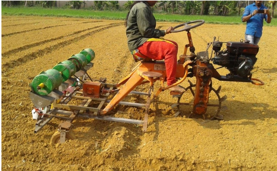
Fig. 4.14 Refined prototype working in the field
