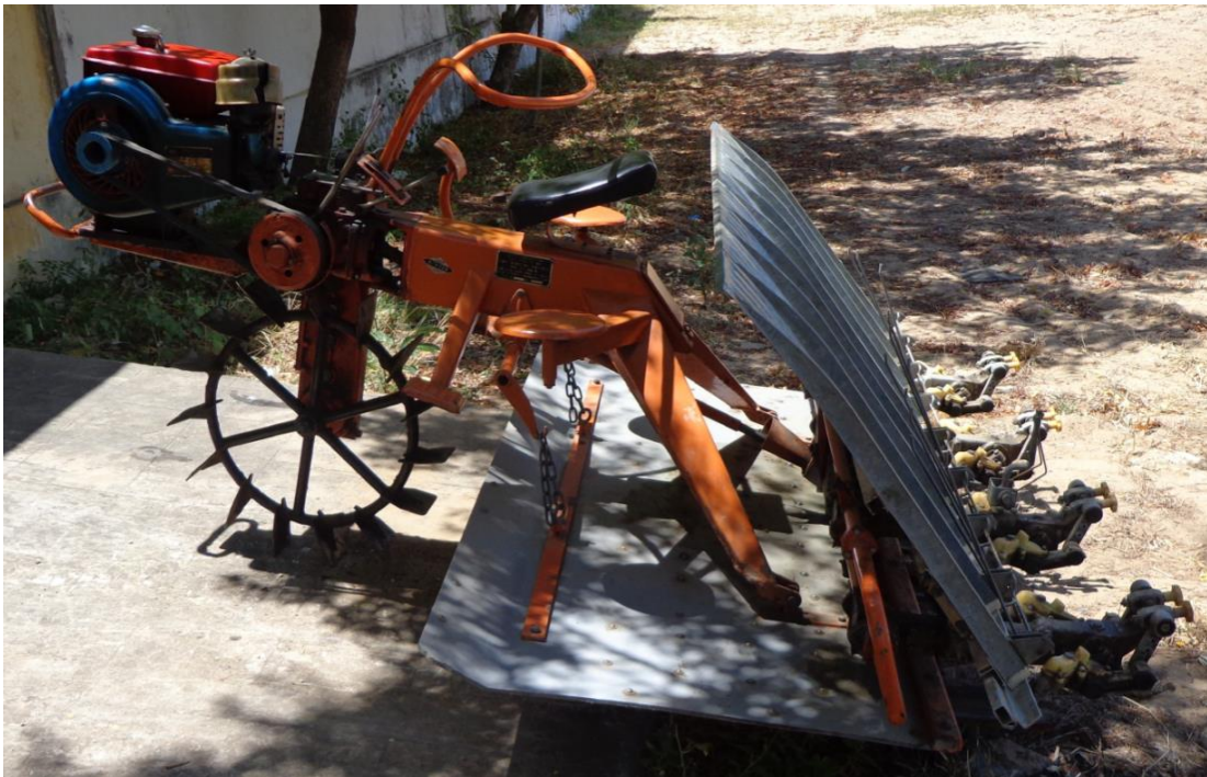
Fig.3.1 Basic model of a Yanji-Sakthi rice transplanter
