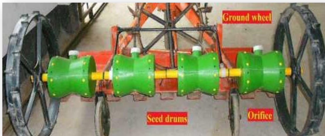
Fig.2.4 TNAU drum seeder mounted to the rear end of machine
