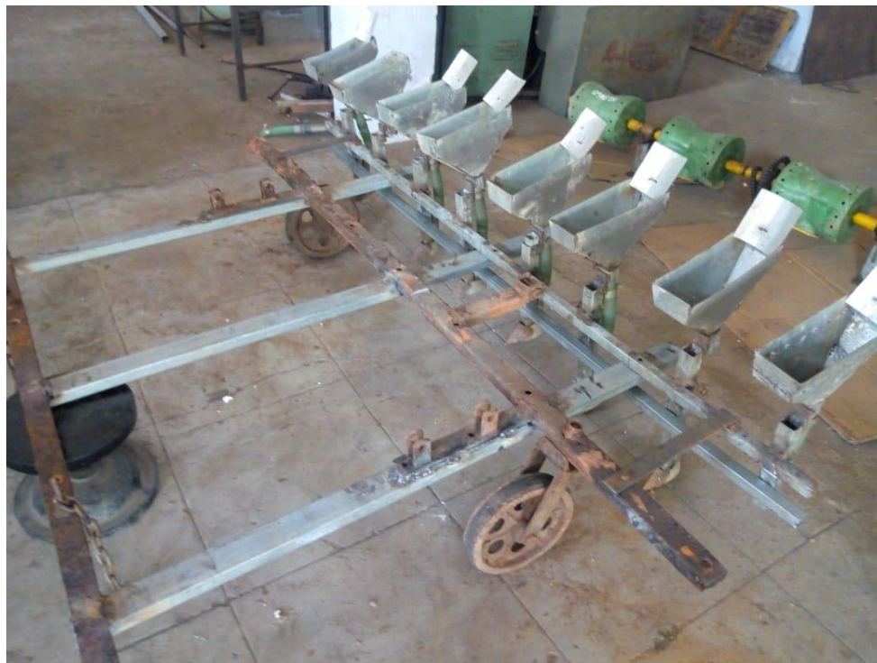
Fig. 4.12 Seeder attachment fitted with modified frame
