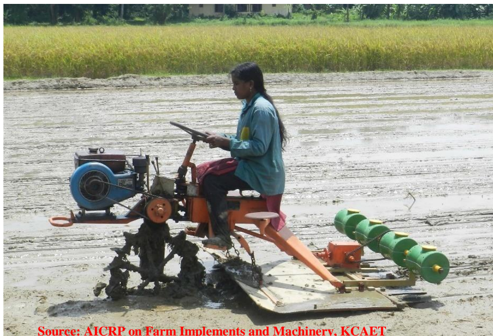
Fig.3.2 Yanji-Sakthi rice transplanter with wet seeding attachment
