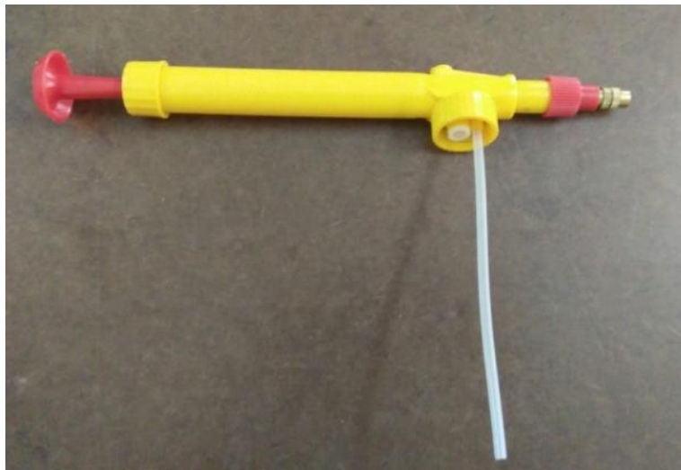
Plate 3.15 Pneumatic hand sprayer
