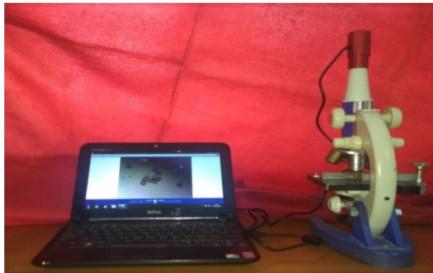
Plate 3.4 Setup for dimension measurements of pollen grains
