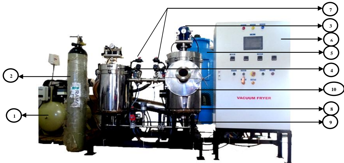
Plate 3.2. Vacuum frying system for bitter melon chips
