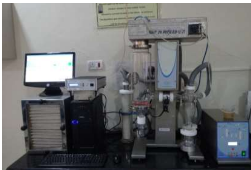
Plate 3.5 Spray dryer used for the production of nanoencapsulated cumin oil powder
