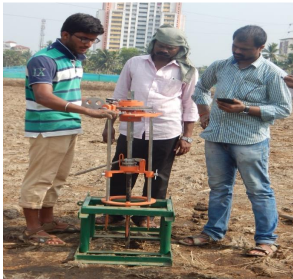
Plate 3.1 In-situ measurement of shear strength
