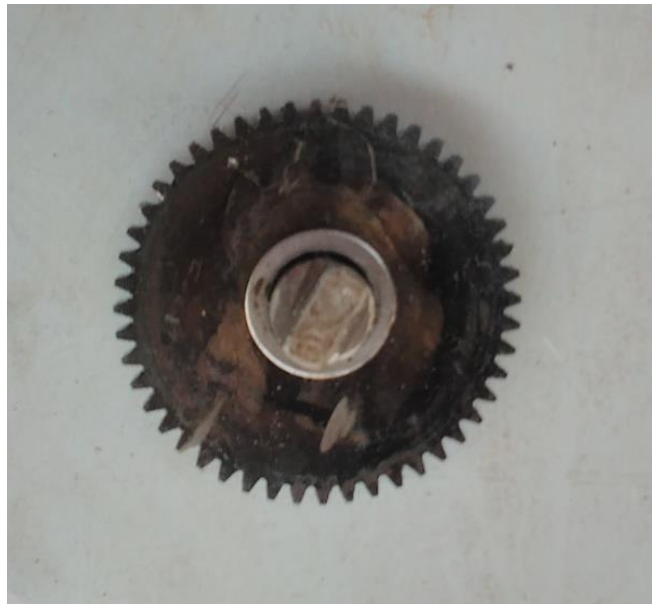
Plate.4.9. Gear with 48 teeth
