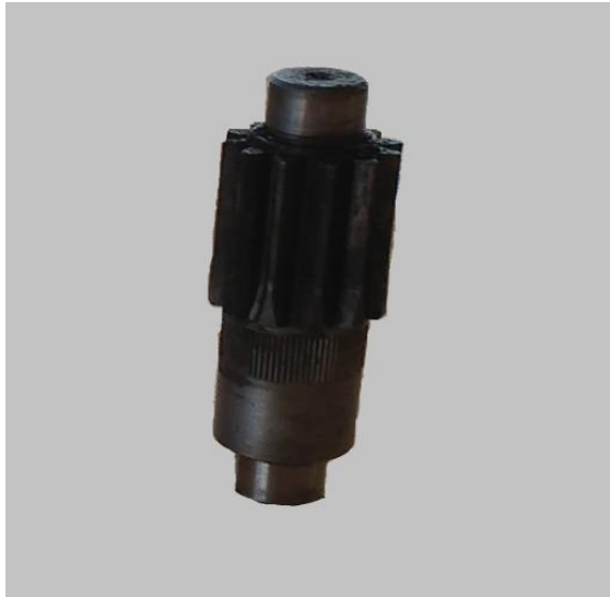
Plate.4.10. Gear with 12 teeth
