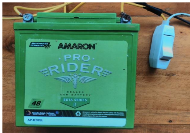
Plate.3.4. Battery with connection cables and switch
