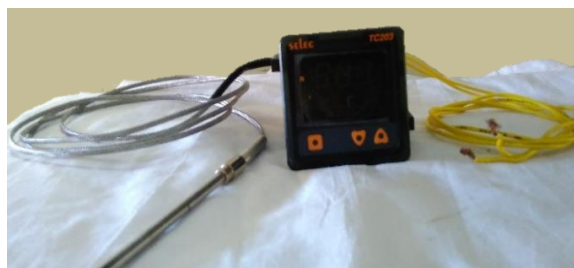
Plate 3.8. Temperature sensor and controller
