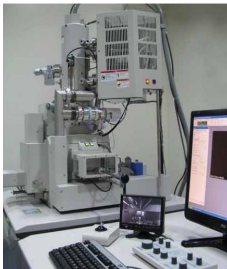
Plate 3.16. Hitachi SU6600 Variable Pressure Field Emission Scanning Electron Microscope (FESEM)
