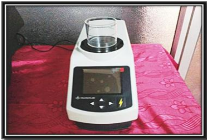
Plate 3.1 Hunter Lab colorimeter
