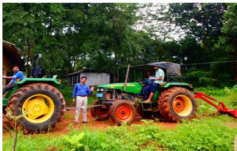
Plate 3.8 Draft measurement of the modified uprooting machine
