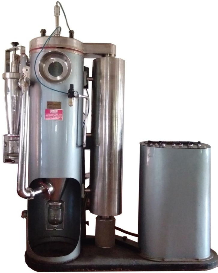
Plate 3.3 Spray dryer used for drying of green tea extract
