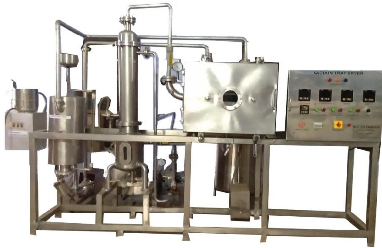
Plate 3.2 Vacuum dryer used for drying of green tea extract
