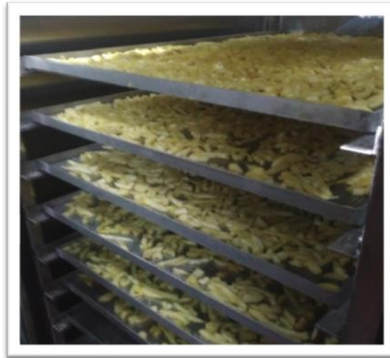
Plate 3.2 Drying chamber with loading of jackfruit sample
