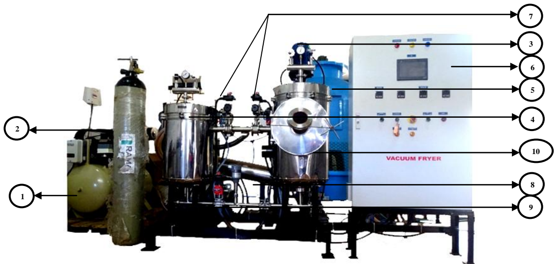
Plate. 3.4 Three dimensional view of vacuum frying system
