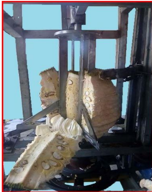
Plate 3.15 Cutting-coring operation of jackfruit
