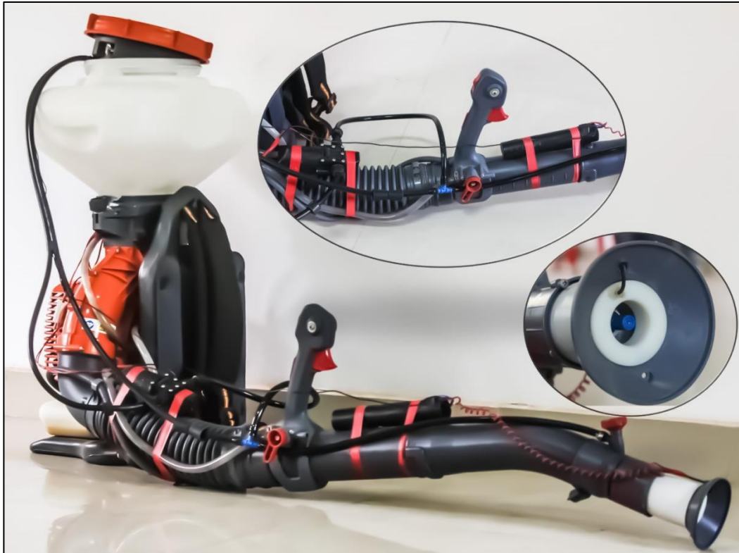
Plate 6. Electrostatic induction charging unit attached to the powered knapsack mist blower
