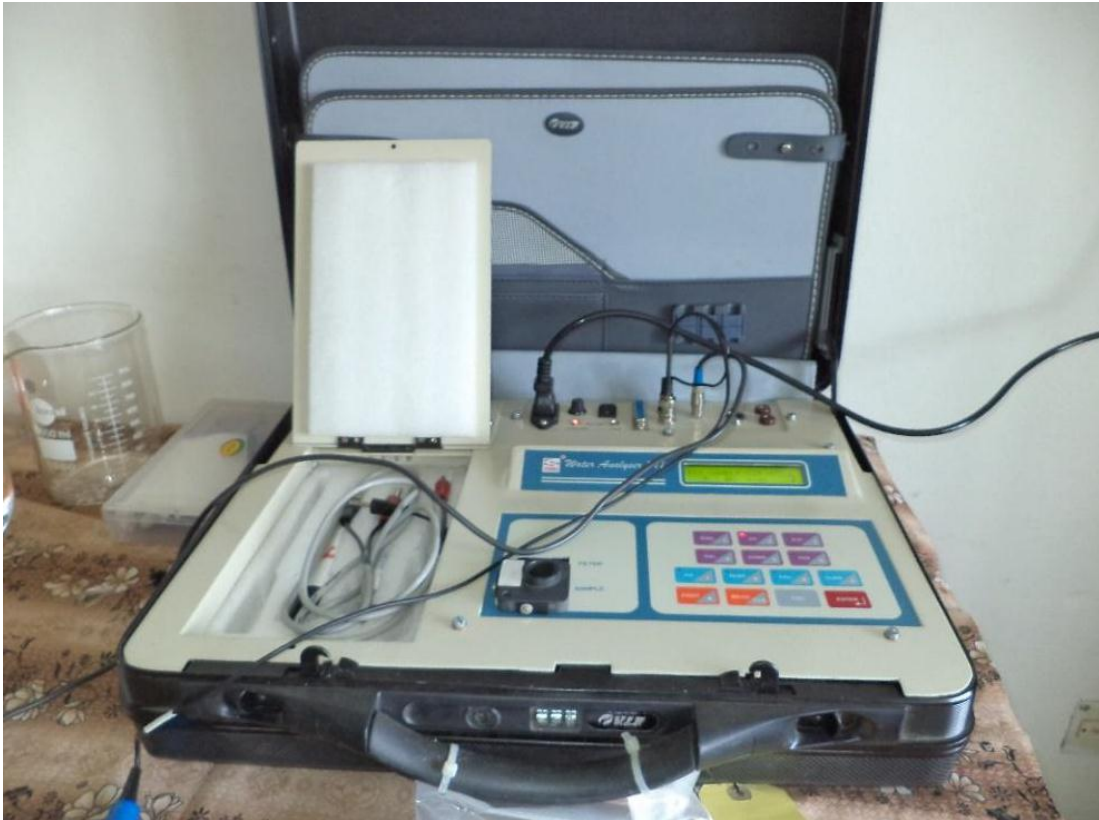
Plate 3.2 Systronics water quality analyzer
