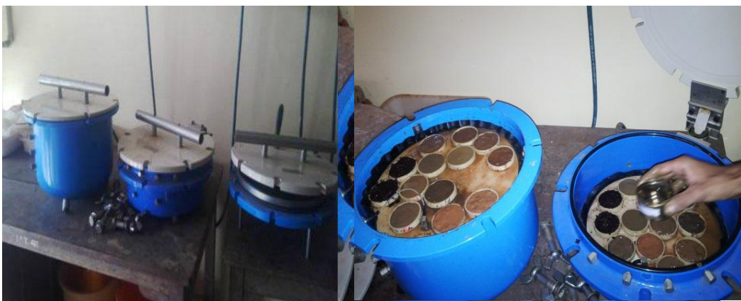
Plate 3.2 Pressure plate apparatus for determination of media moisture retention characteristics
