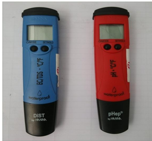
Plate 3.3 Digital EC and pH meter
