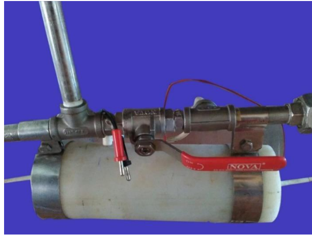
Plate 3.2 Ohmic heating chamber
