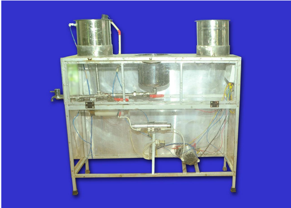
Plate 3.1 Developed combined Ohmic heating and UV treatment apparatus
