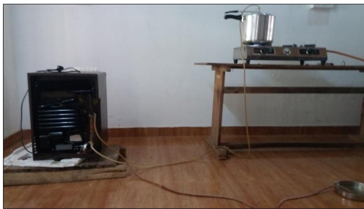
Plate 3.7 Setup for the performance of VARS using hot water generated in a steel vessel
