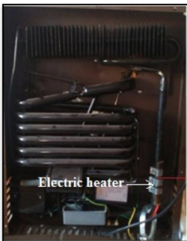
Plate 3.9 VARS with Electric heater
