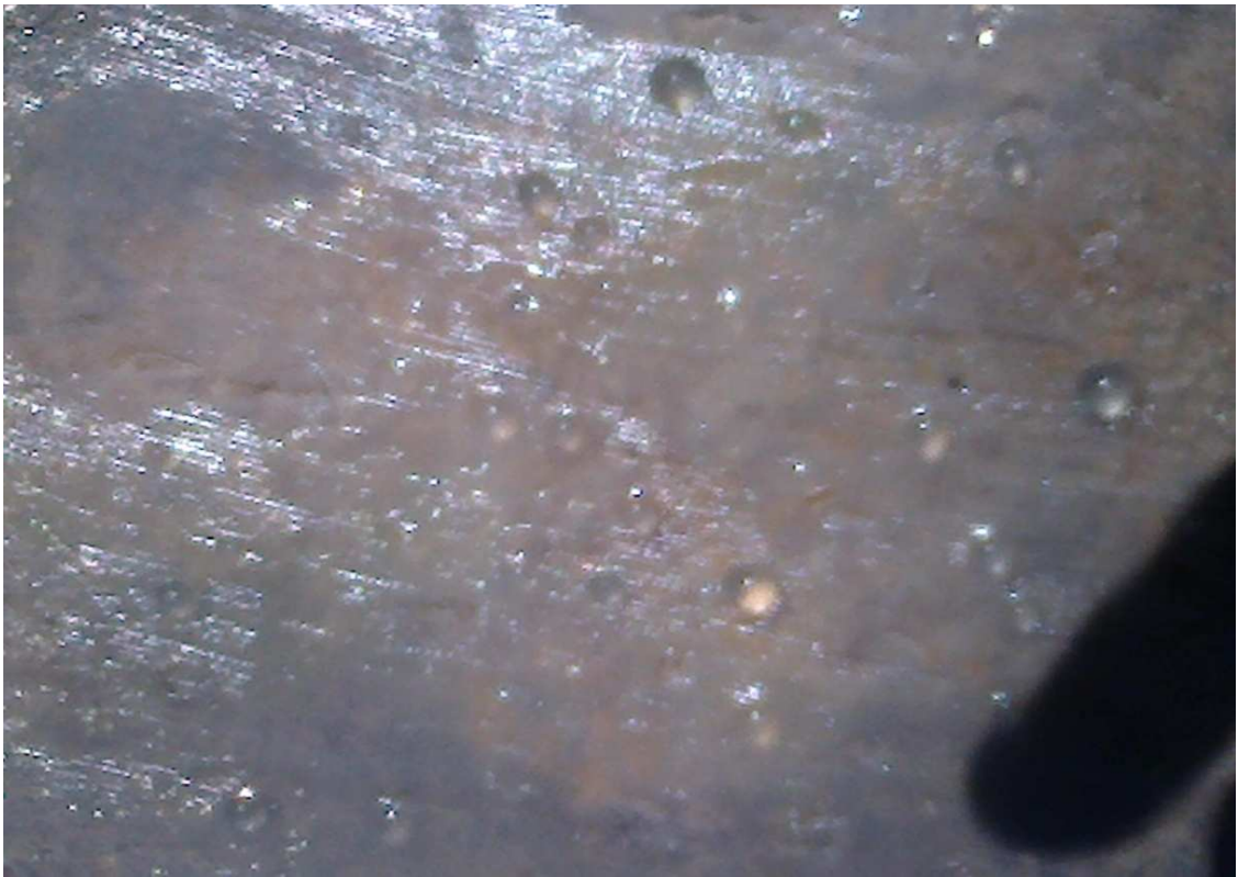
Plate 6. Testing for average drop size of simulated rainfall
