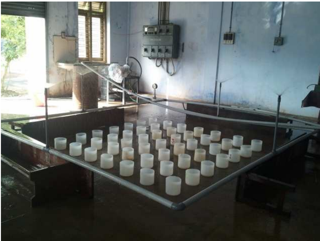
Plate 5. Rainfall simulator testing
