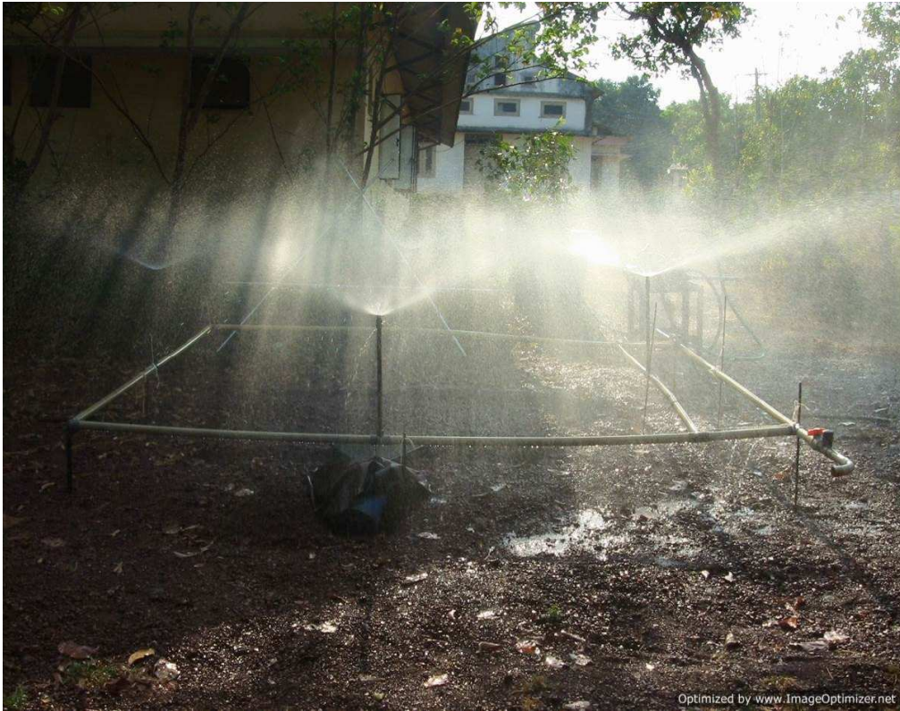
Plate 8. Rainfall simulator in operation on erosion plot
