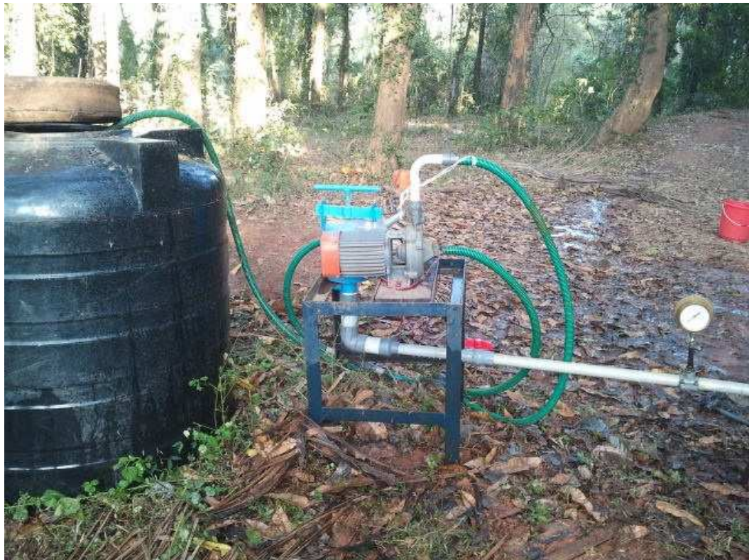
Plate 4. Water supply to the rainfall simulator
