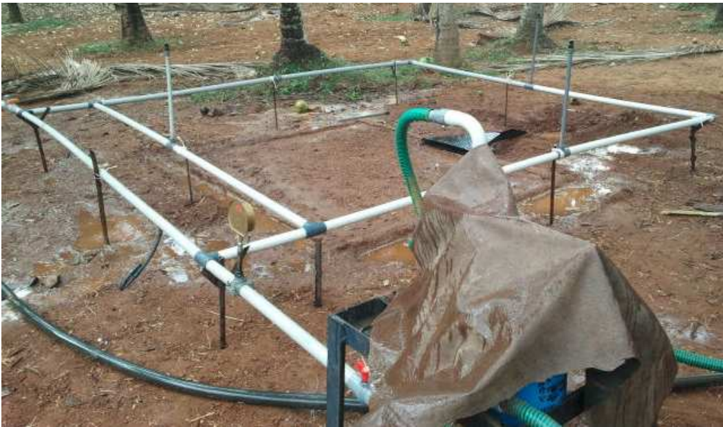
Plate 1. Installation of rainfall simulator on micro plot
