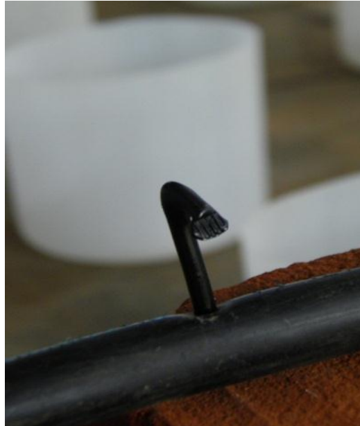
Plate 3.5 Micro sprinkler with lateral
