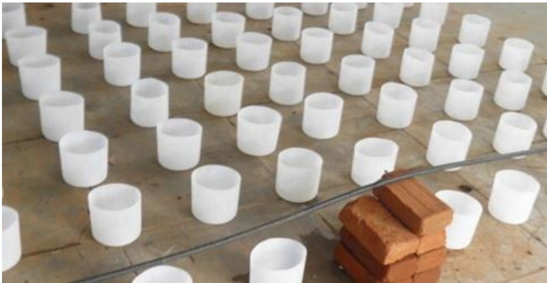
Plate 3. 6 Uniformity test using catch cans
