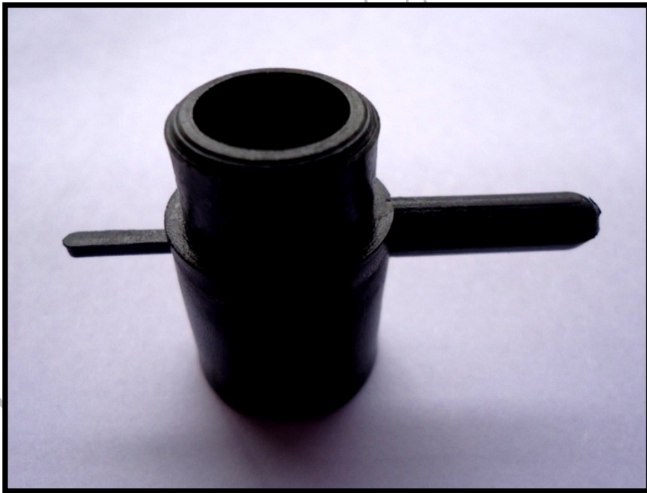
Plate 4.6 Bottom part of the emitter
