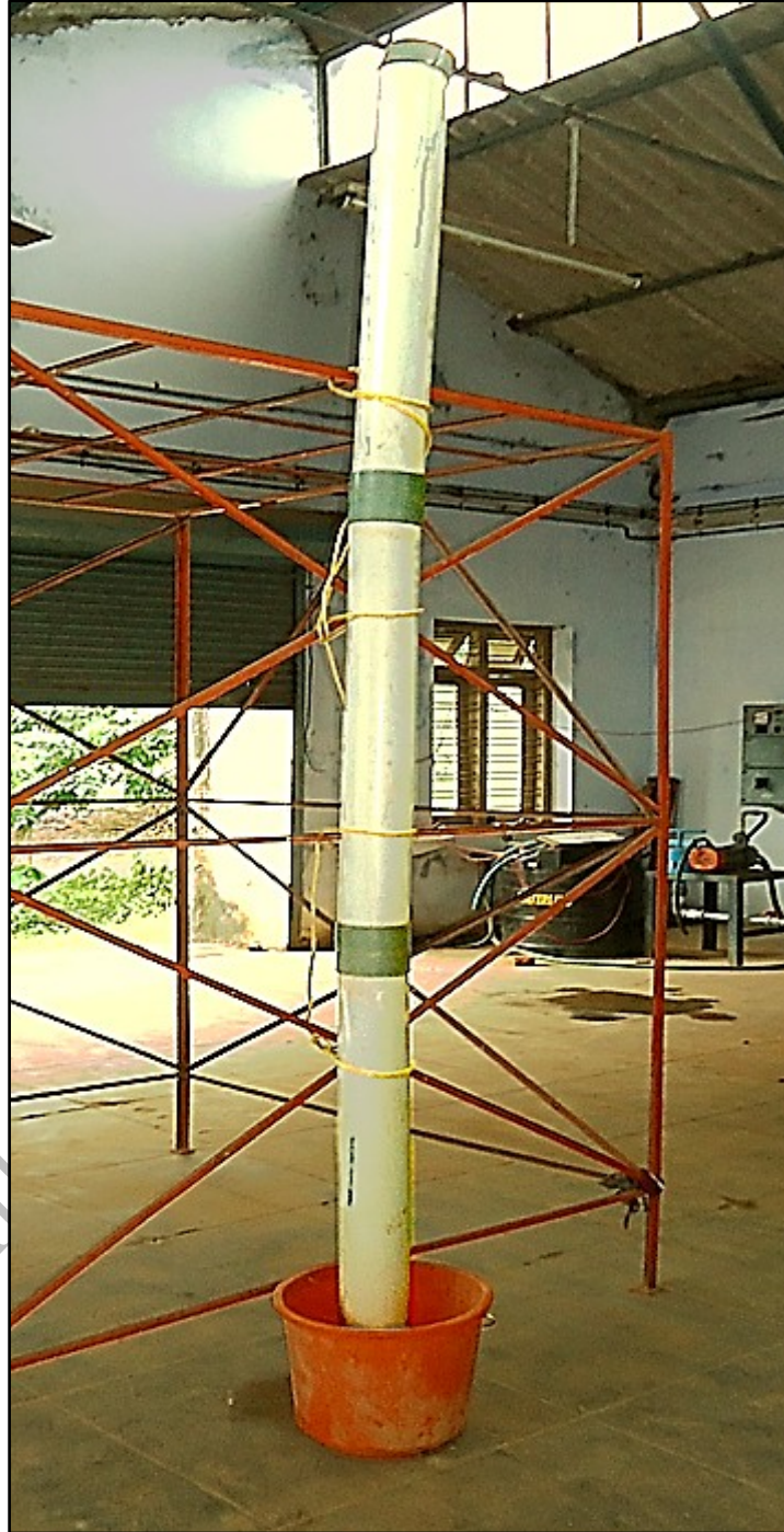
Plate 3.1 Experimental setup for determining the Wetting Curve
