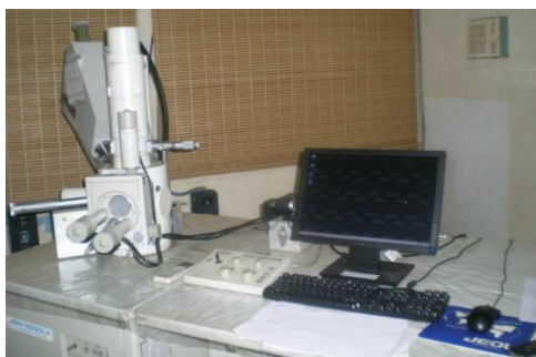
Plate 3.6 JEOL JSM 5600LV Scanning Electron Microscope for particle size analysis
