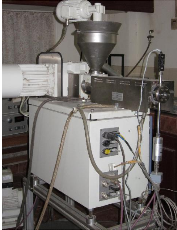
Plate 3.3 Brabender single screw extruder
