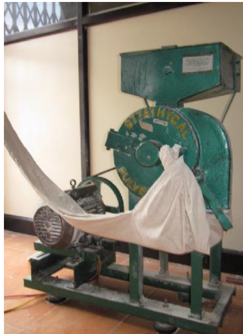
Plate 3.2 Hammer mill (Mimac)
