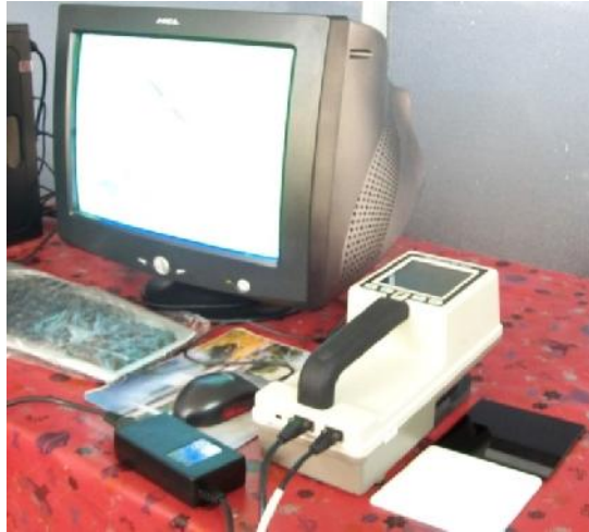
Plate 3.11 Experimental set up of Hunter lab colour flex meter
