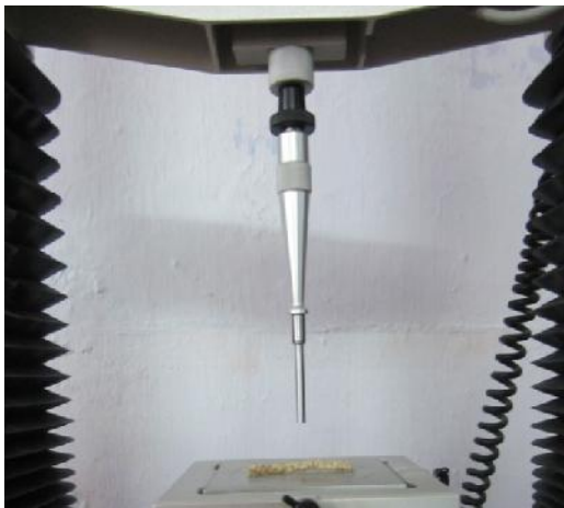
Plate 3.10 Probes for Compression (5mm Stainless steel cylindrical probe) and Snap Test (three point HDP/3PB bend rig)
