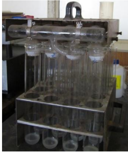
Plate 3.16 Kjeldahl digestion tubes in protein digester
