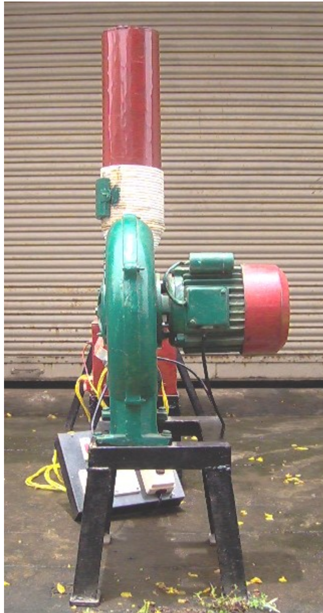
Plate 3.3 Nutmeg mace dryer- Side view
