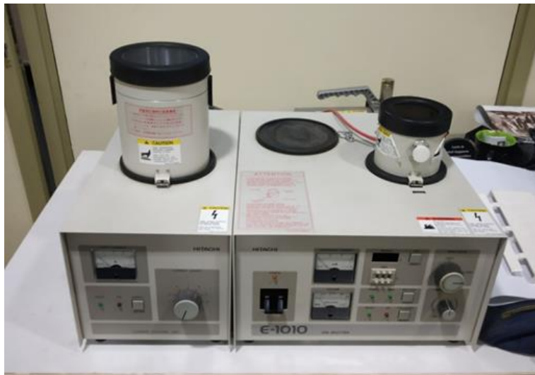
Plate 3.15 Ion sputter coating unit
