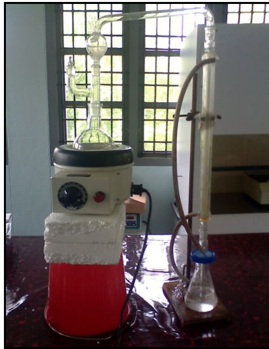
Plate 8 Experimental set up for distillation in determination of TKN.
