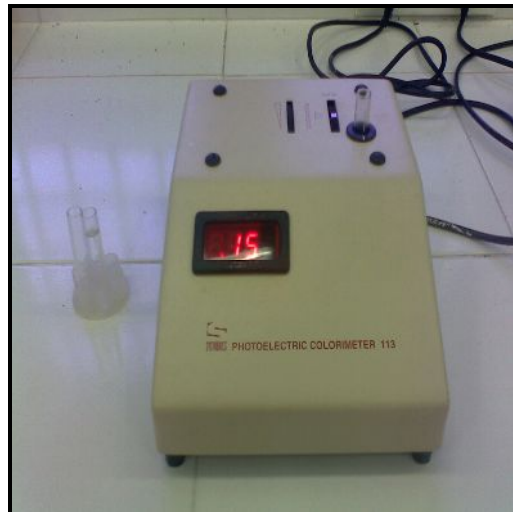
Plate 10 Photoelectric colorimeter used for determination of Phosphate.
