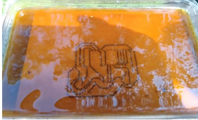
Fig 3.24 Printed Copper Clad dipped in \text{FeCl}_3 Solution
