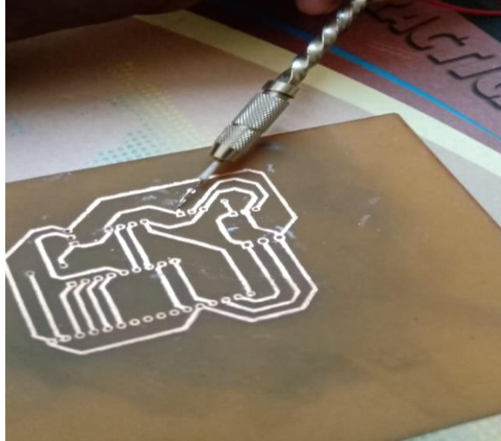
Fig 3.26 PCB board drilling
