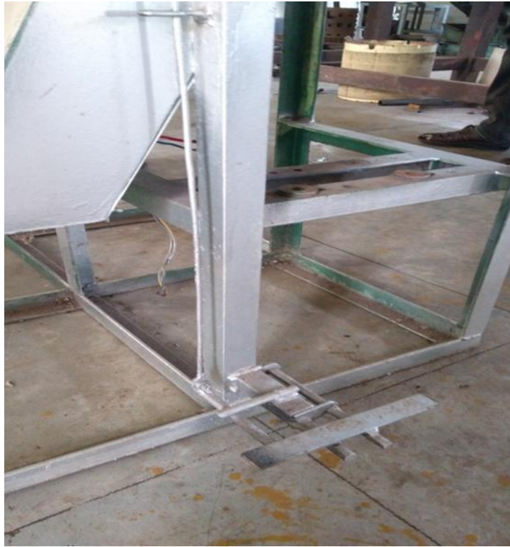
Plate 4. Pedal operating portion of feed pressing mechanism
