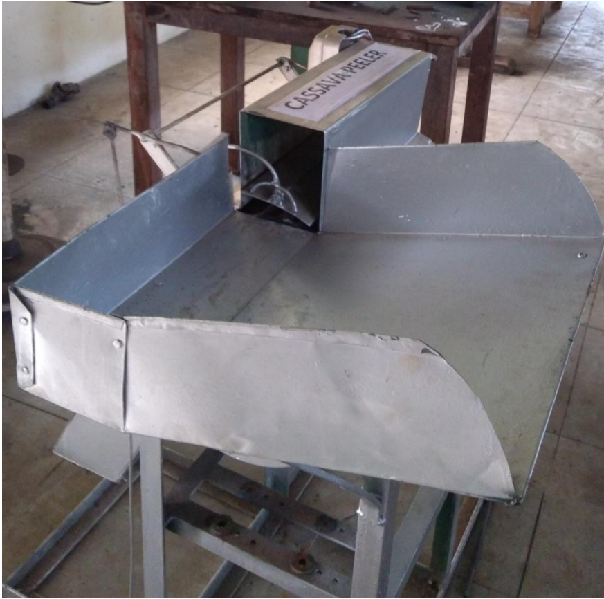
Plate 3. Feed pressing mechanism top portion
