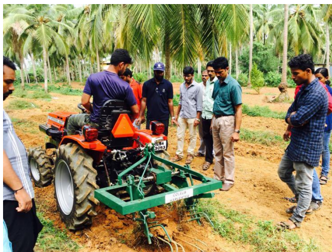
Plate 3.4 Field testing of mini tractor operated coleus digger
