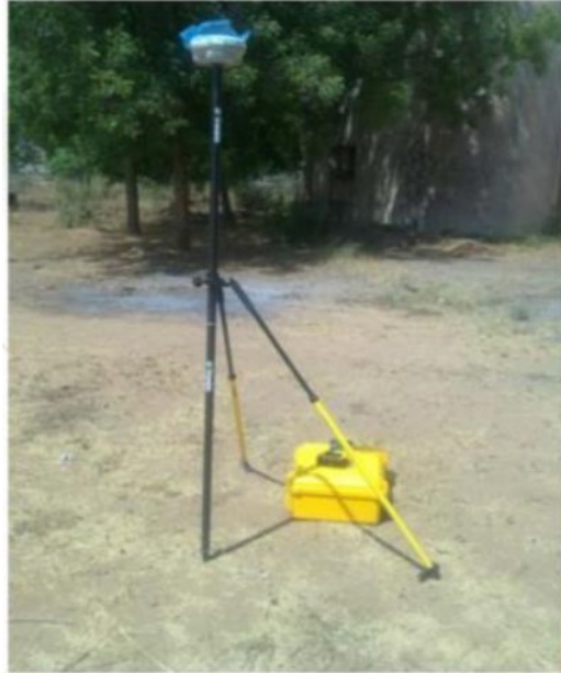
Plate 3.3 Rover setup in PPK survey
