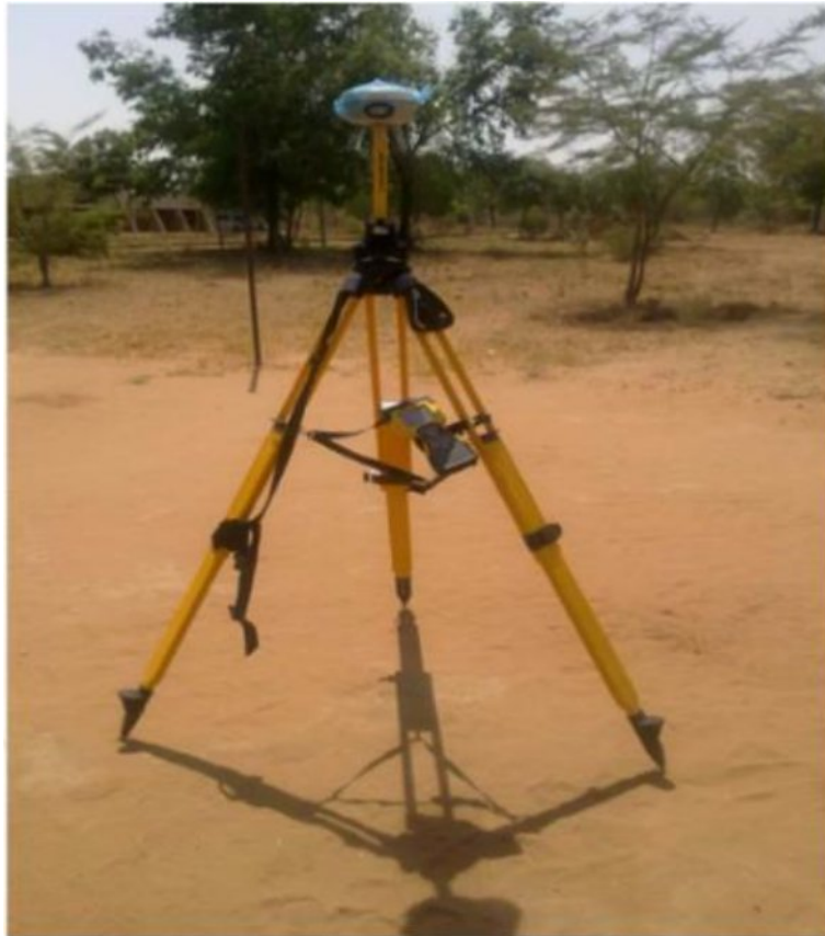
Plate 3.2 Base setup in PPK survey
