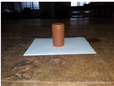
Plate 4.1 UCS soil sample-1 from the mould (without reinforcement)
