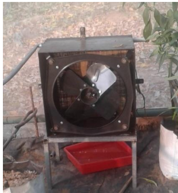
Plate 3.2 Box type fan and pad cooling system (type B)
