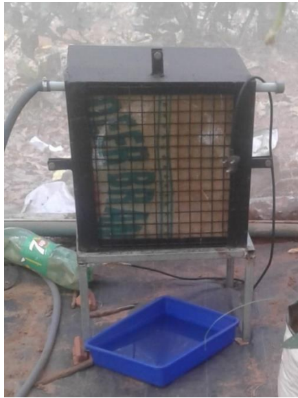
Plate 3.1 Box type fan and pad cooling system(type A)
