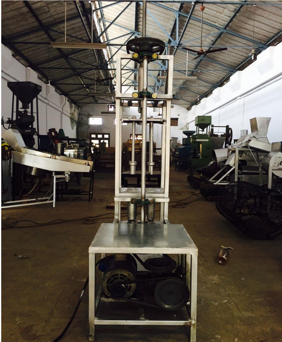
Plate 3.1. Power Operated Plantain Peeler
