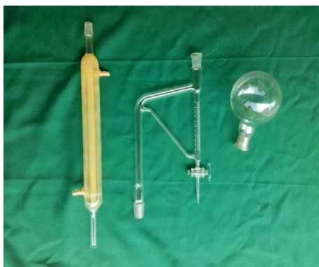
Plate 3.2. Components of the extraction system
