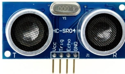
Fig 3.4 HC SR04 Ultrasonic Sensor
