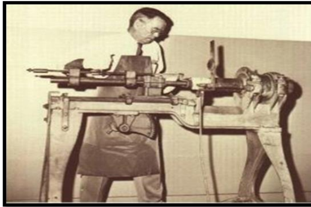
Fig. 2.6 Basic model of Ginaca machine (The American society of mechanical engineers, 1993)
