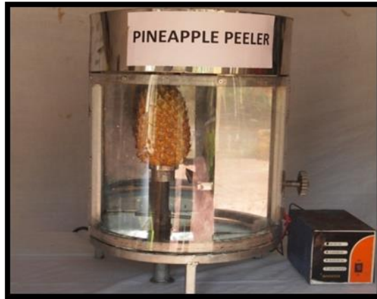
Plate 3.8 Pineapple peeling machine
