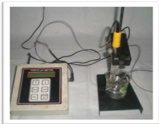
Plate 3.3 YORCO pH meter, model: YSI – 601
