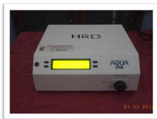
Plate 3.4 Aqua lab water activity meter
