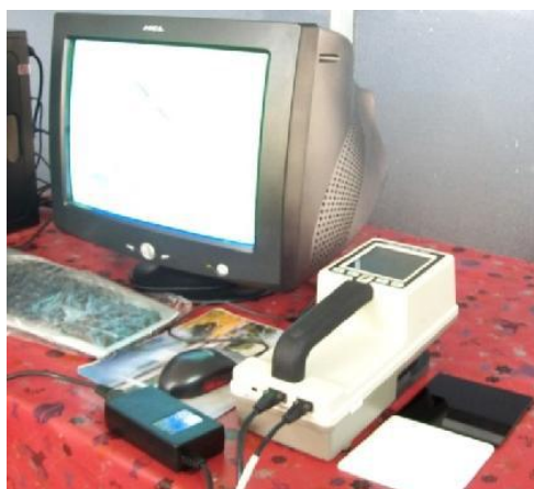
Plate 3.3 Experimental set up of Hunter lab colour flex meter
