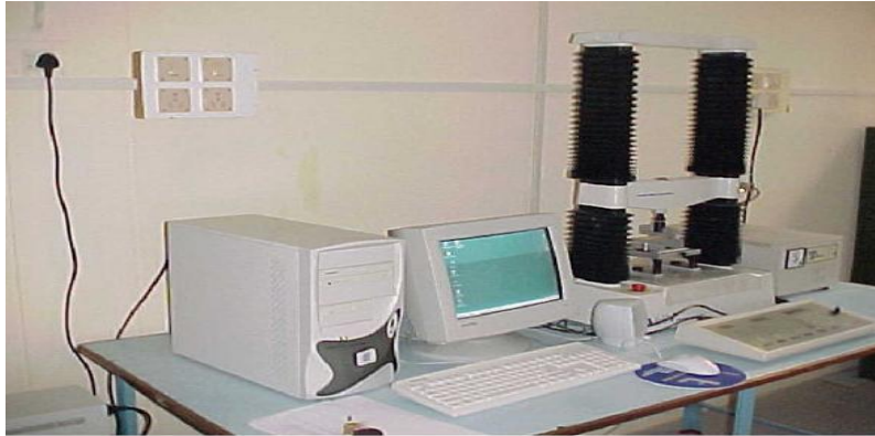
Plate 3.4 Experimental set up of TA.XT plus texture analyser
