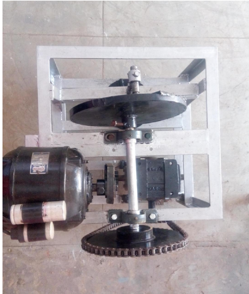
Plate3.11. Top view of chapati pressing machine
