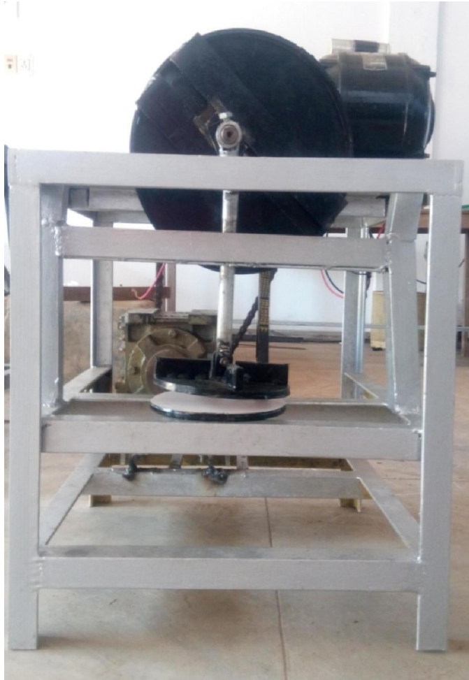
Plate3.10. Side view of chapati pressing machine
