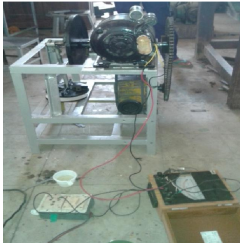
Plate4.1. Watt meter connected to the machine
