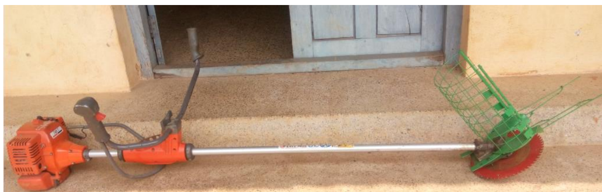
Plate 3.5 Brush cutter with holder attachment
