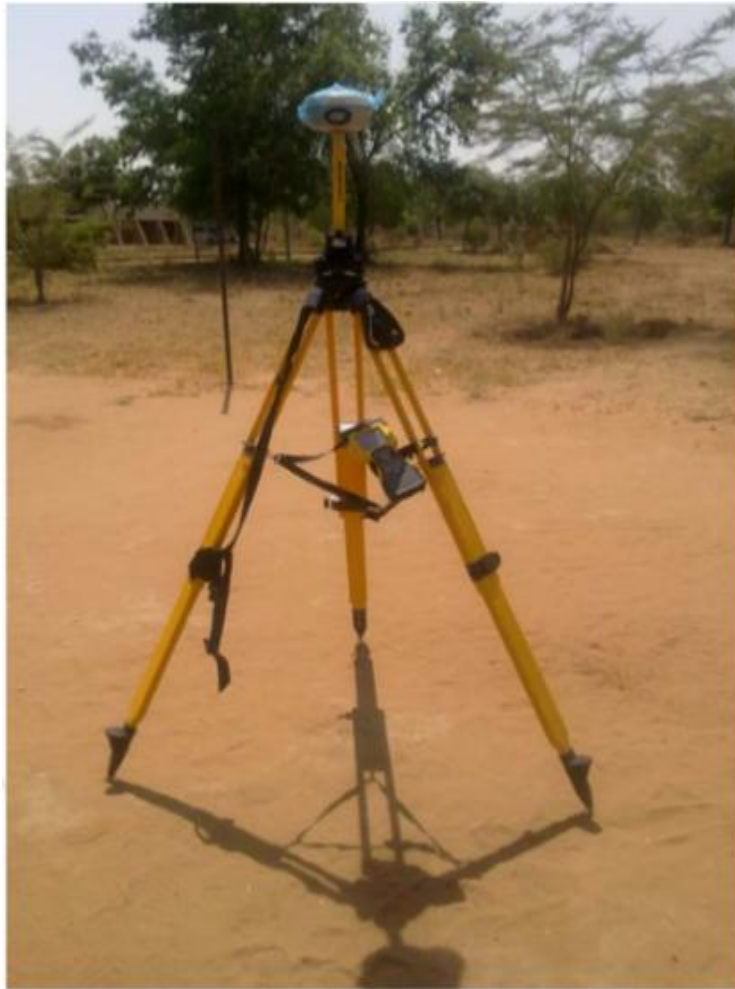
Plate 3.6 Base setup in PPK survey
