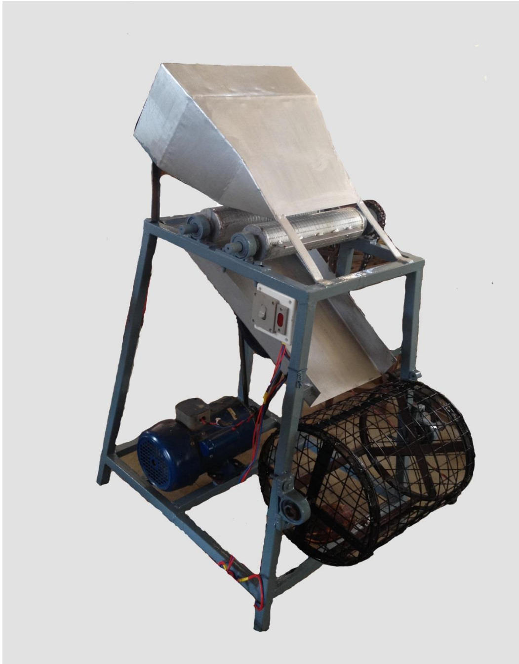
Plate 3.6 Cocoa pod breaker cum bean extractor
