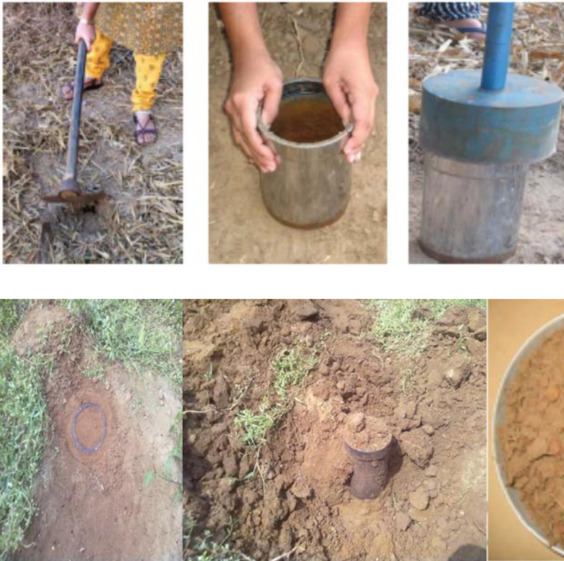
Plate 3.2 Sampling by core cutter
